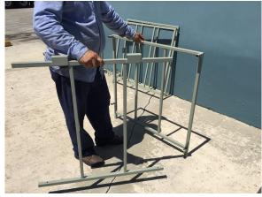
**Step Two:** Join one of the two side panels with the long panel by sliding both of the panels bars together.
