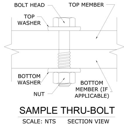
Note: The term "Thru-Bolt" or through bolt, if used herein, refers to a bolt passing through the member(s) in contact and is fastened by a nut at the end opposite the screw head. Nut shall be equivalent to or exceed the strength of the bolt U.N.O. Nut shall be sized to accommodate the same nominal diameter as the bolt U.N.O. See diagram above-right for a sample thru-bolt configuration.
