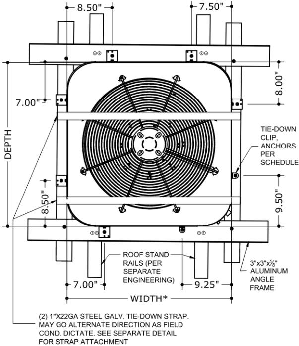
\*NOTE: FOR CONDITIONS WITH STAND DEPTH GREATER THAN UNIT DEPTH, MIAMI-TECH SUPPORT ANGLES (PART #AS14CABBXX) PER NOA#17-1218.02 SHALL BE PROVIDED OR SITE-SPECIFIC ENGINEERING IS REQUIRED.
