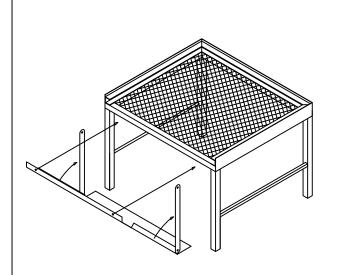
AFFIX TO STAND WITH PROVIDED #10 SELF-TAPPING SMS. SCREW TWO THROUGH THE FRONT PANEL, AND ONE THROUGH EACH SIDE ARM ON THE UNDERSIDE OF THE STAND.
